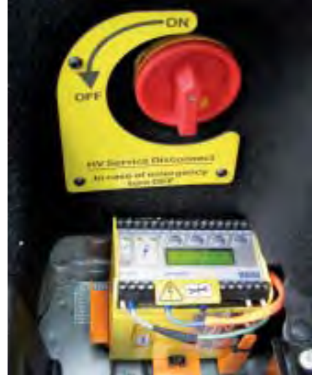
The Bender A-ISOMETER® of type IRDH275W-4925 is under a cover in the boot.
